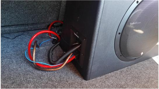
13. If installing the RF Punch sub, attach the volume/gain remote and run it under the driver's side trim panels just like you did with the power cable on the passenger side (this will be much easier, as the wire is smaller). 14. Adjust your gain, crossover frequency, etc. Enjoy.
