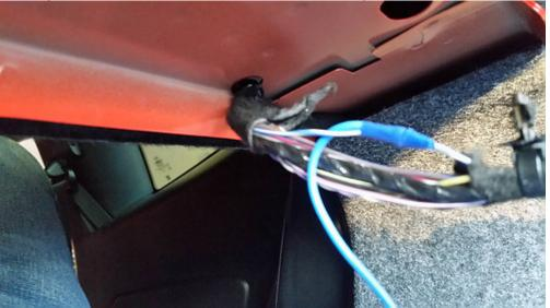
6. If you plan on using the 12V switch wire to signal your amp to turn off and on, then repeat steps 2 through 5 for that wire. Be careful not to break the
