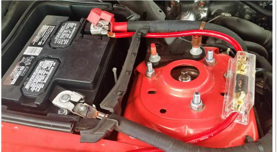
12. Attach the other end of the short cable to the fuse. Make sure it's tight. 13. Attach the end of the long cable to the fuse. Make sure it's tight.
