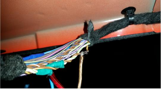
5. Wrap the soldered connection with electrical tape:
