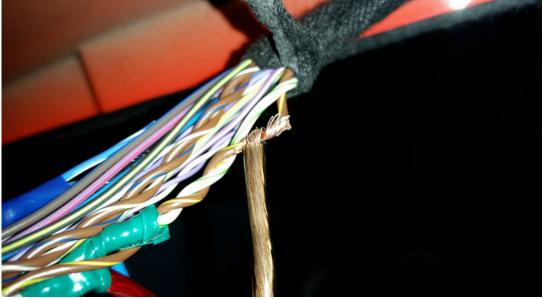
I then soldered them together (I don't recommend tinning the new wire first, as that will make it near impossible to wrap it around the existing Ford wire):
